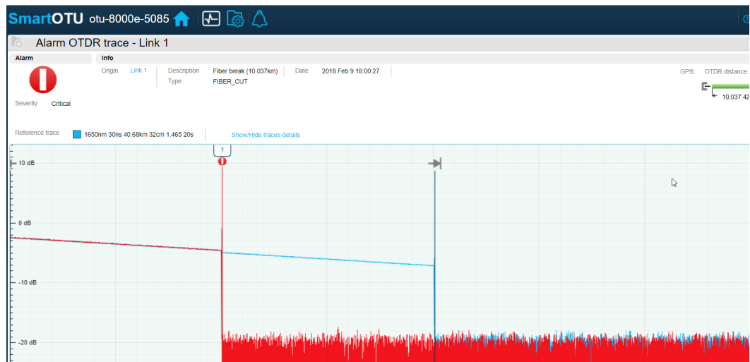
Figure 32 Fiber Cut - Critical Alarm on connector
