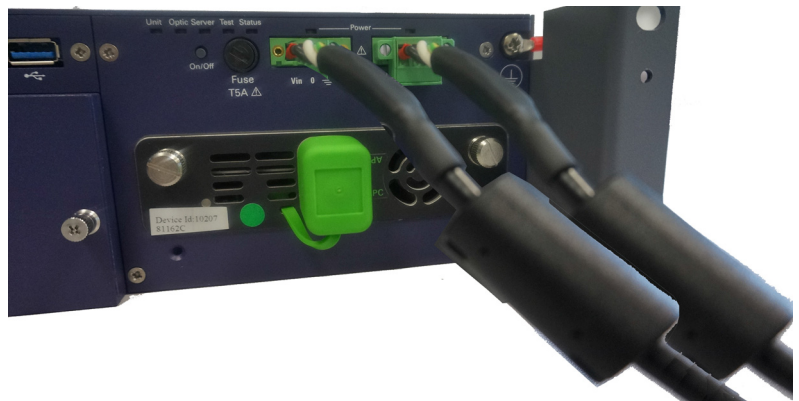
Figure 13 Dual power feed installed on front frame
