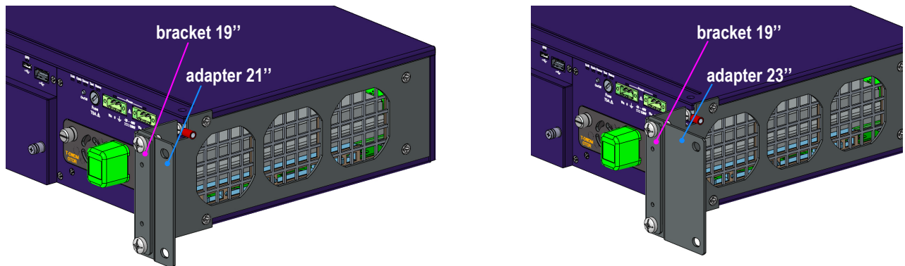
Figure 10 Fixing the 21" or 23" adapters (optional) onto the 19" brackets
