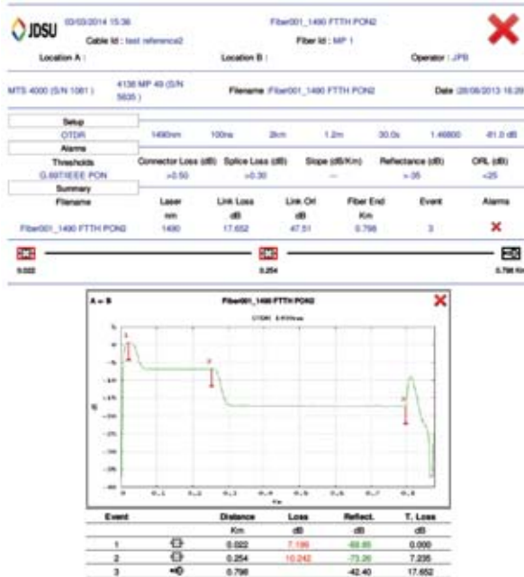
Figure 92 Fast Report with FTTH-SLM option
