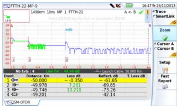
Figure 84 FTTH OTDR Trace
