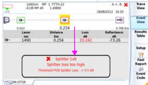
Figure 89 SmartLink: Event View
