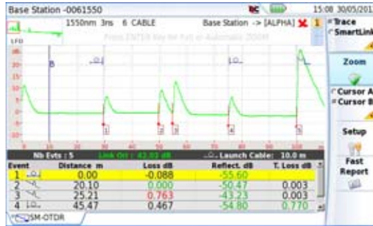
Figure 71 FTTA OTDR Trace
