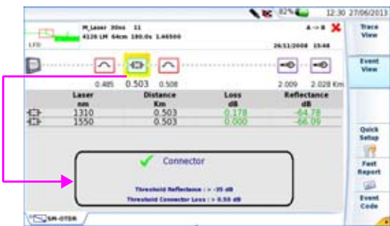
Figure 49 SmartLink: Event View
