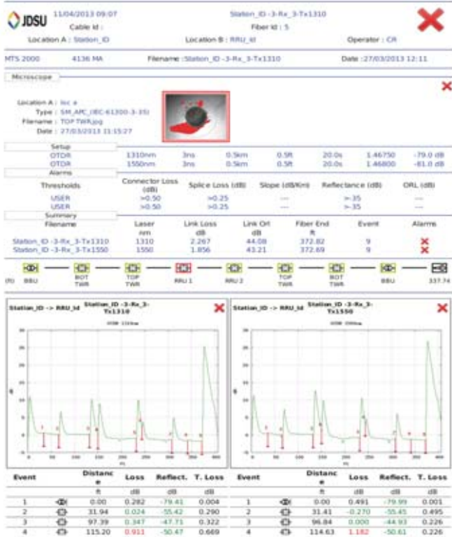
Figure 79 Fast Report with FTTA-SLM option
