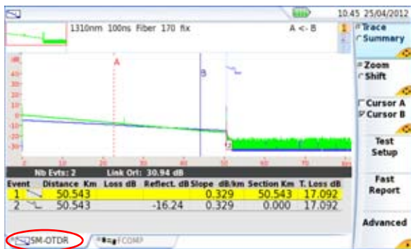
Figure 123 OTDR trace
