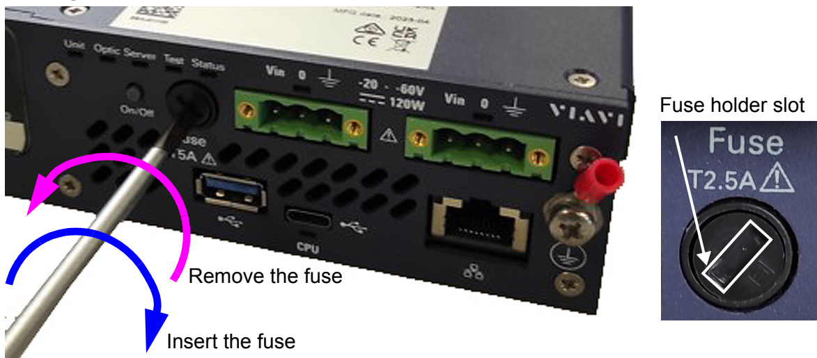
Figure 48 Remove/Insert the fuse
