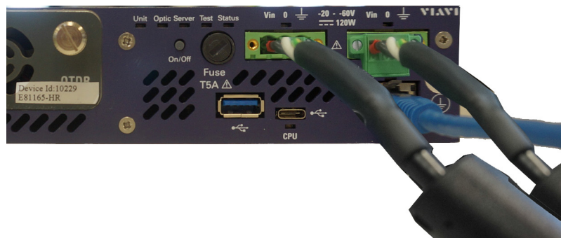
Figure 14 Dual power feed installed on front frame
