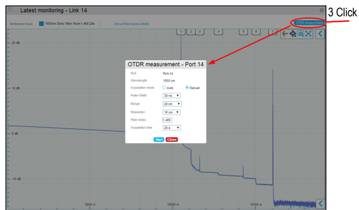
Figure 30 OTDR measurement
