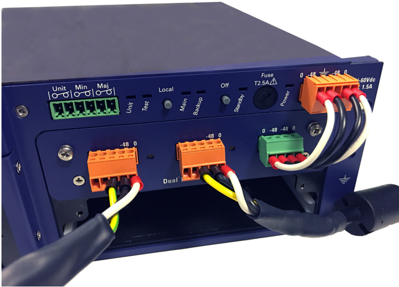
Figure 23 Wiring for Dual power feed
