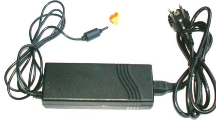
Figure 5 Converter with female connector delivered
