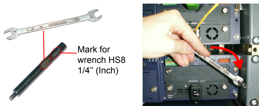
Figure 20 Spacer onto the OTU-8000
