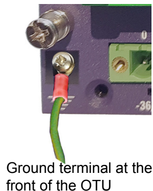
Figure 16 Ground Connector
