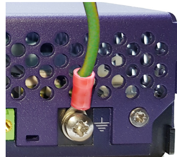
Ground terminal at the rear of the OTU
