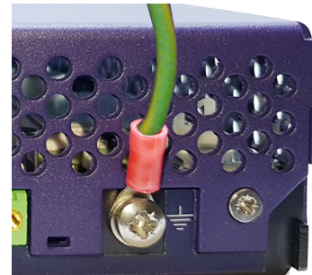
Ground terminal at the rear of the OTU
