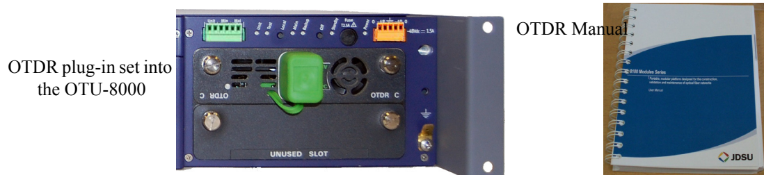
Figure 15 OTDR Module mounted + User Manual
