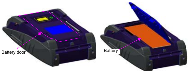
Fig. 91 Battery installation
