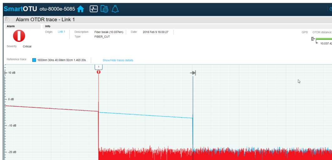
Figure 32 Fiber Cut - Critical Alarm on connector
