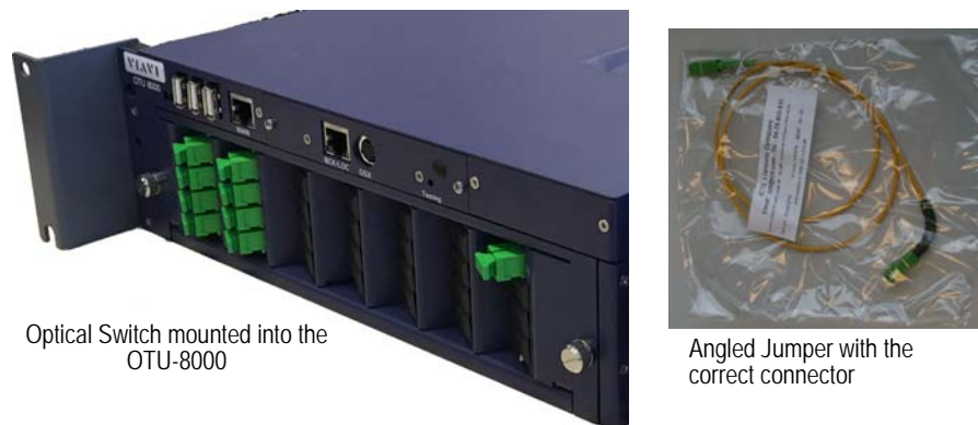
Figure 10 Optical Switch module set into the OTU-8000 and angled jumper
