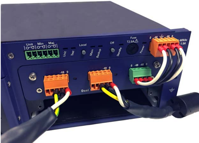
Figure 23 Wiring for Dual power feed
