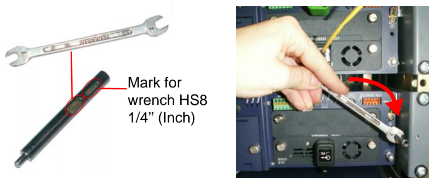
Figure 20 Spacer onto the OTU-8000
