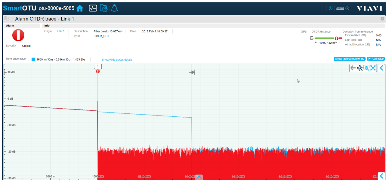
Figure 33 Fiber Cut - Major Alarm
