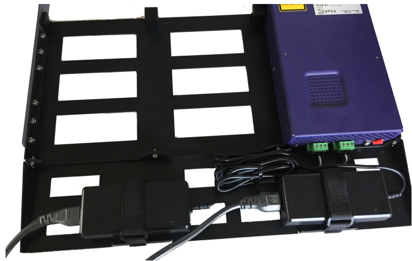
Figure 15 Dual power feed installed on rear frame
