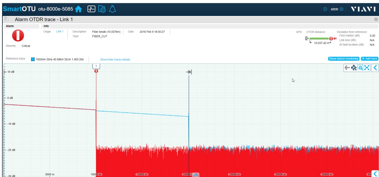
Figure 33 Fiber Cut - Major Alarm
